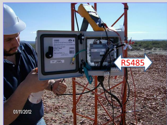
Figure 4 – Deployment of DIN-RS485 board in DIN-rail cabinet with METEO units in Cutral-C6 (Neuquén) Small Wind Turbine Test Site
