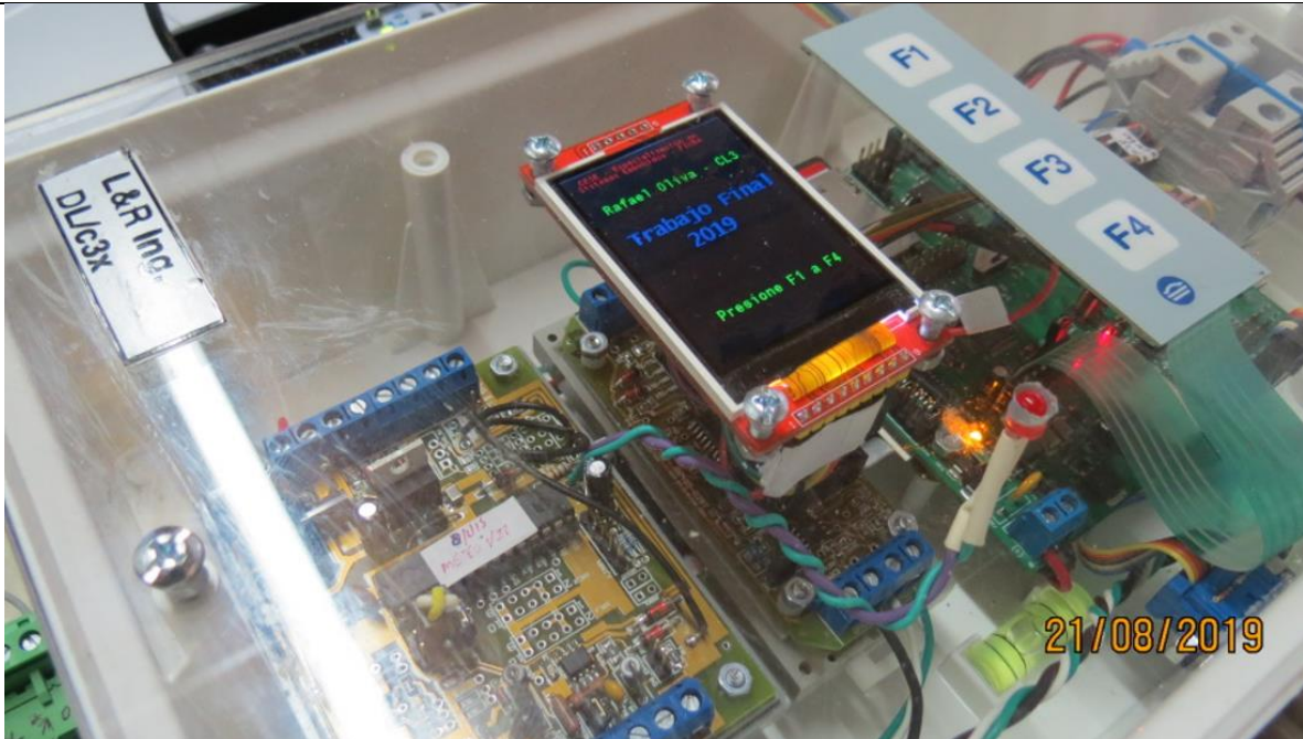
Figure 7a – Connection of CL3 and METEO board using DIN-RS485 board operating in TTL to RS485 Mode
