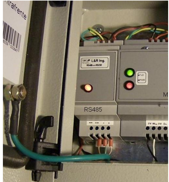
Figure 3 – One of the possible applications – Diagram of DIN-RS485 board serving as link between METEO units and PWRC2 (CL2) SWT-Power Curve Data Loggers
