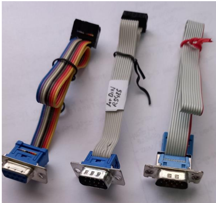
Figure 6 – RS232 side cables using standard 0.1" crimp female IDC connectors to flat cable and either male or female DB-9 connectors
